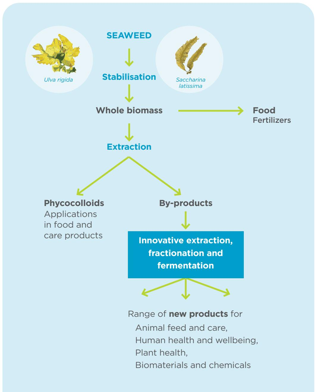
Figure 5 Processes and products of seaweed biorefinery. Graphic designed by AquaTT.
