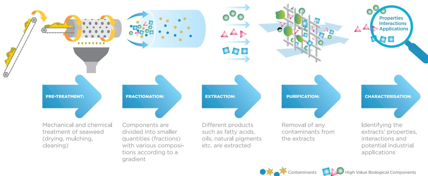
Figure 6 Steps of the biorefinery process. Graphic designed by AquaTT.
